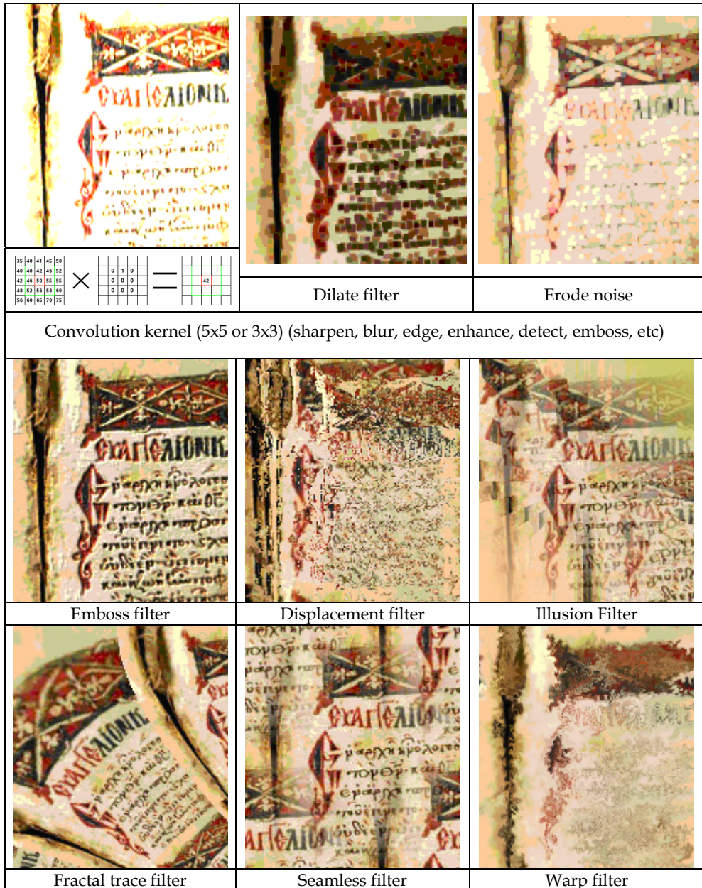
Fig. 31. Convolution filters / Erosion / Dilation on Images
